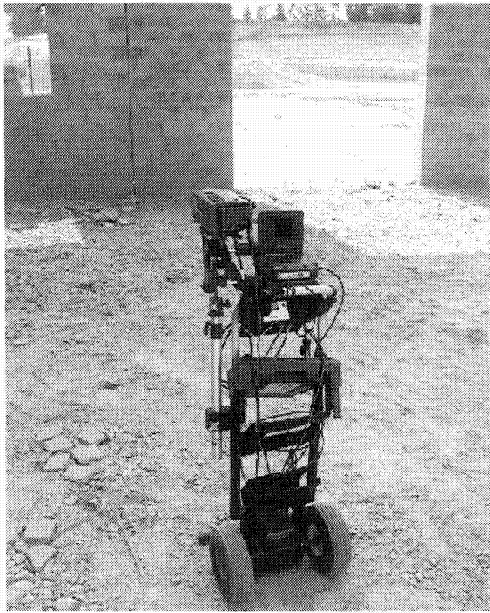
Figure 12) Photograph of a cart-mounted 390 ThermaCAM™, with continuous recording system
